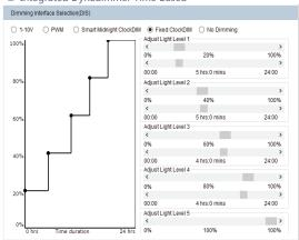
Allow users to separate 24hrs into 5 sections and corresponding output current.
