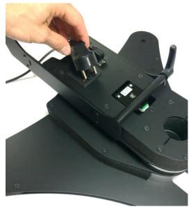
The maximum current supported by the lamp output is 3A, which is 660 W at 220 VAC and 330 W at 110 VAC.
